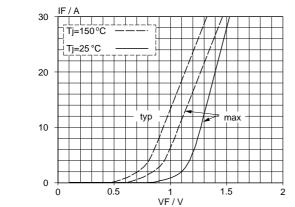
Fig.8. Modulator typical and maximum forward characteristic;  $I_F = f(V_F)$ ; parameter  $T_i$
