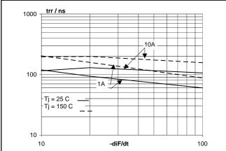
Fig.9. Modulator maximum  $t_{rr}$  measured to 25% of  $I_{rrm}$ ;  $T_j = 25^{\circ}\text{C}$  and  $150^{\circ}\text{C}$
