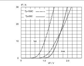
Fig.11. Damper forward characteristic  $I_F = f(V_F)$ ; parameter  $T_i$
